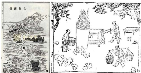
Illustrations from Tiangong Kaiwu , showing (a) Mining copper ore; (b) smelting copper ore and the process of removing lead elements
