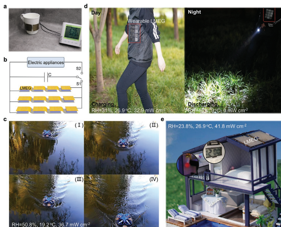
Figure 5. Demonstration of LMEG as practical power source in real life conditions. a) The f-LMEGs bent around a cup could power a temperature-humidity monitor. b) The circuit diagram for applications in (c) and (d). S1: twelve LMEGs in series-parallel connection charging for a capacitor. S2: accumulated energy in the capacitor powering commercial electronics, such as a boat or a flashlight. c) A small speedboat is sailing on the water driven by an LMEG-charged capacitor. d) Left: LMEGs are integrated with garment and charged a capacitor during the day. Right: the electricity stored in the capacitor could light up a flashlight at night. e) LMEGs are installed on the roof of a house model for powering common electronics such as a red LED and an electronic clock in a real natural environment without any other auxiliaries.
